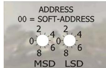
With the ADDRESS switch, the instruments address can be set. The MSD is the high part of the decimal number and the LSD the low part. For instance address 25 means MSD on 2 and LSD on 5. The default switch position is 00. In this position the address is software programmable. The default software programmable address is 1.
